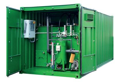
The purification mechanism of modular systems of wastewater treatment Facet SMS Series is based on a biological process of active sludge with extended aeration: the microorganisms in the biomass purify the water, so that no additional chemical treatment throughout the process is necessary.
